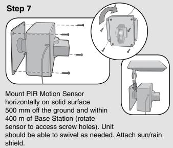
**NOTE:** Keep PIR Motion Sensor antenna away from metal objects. Do not mount PIR Motion Sensor in direct sunlight, near moving tree branches, or in the path of a sprinkler system.
